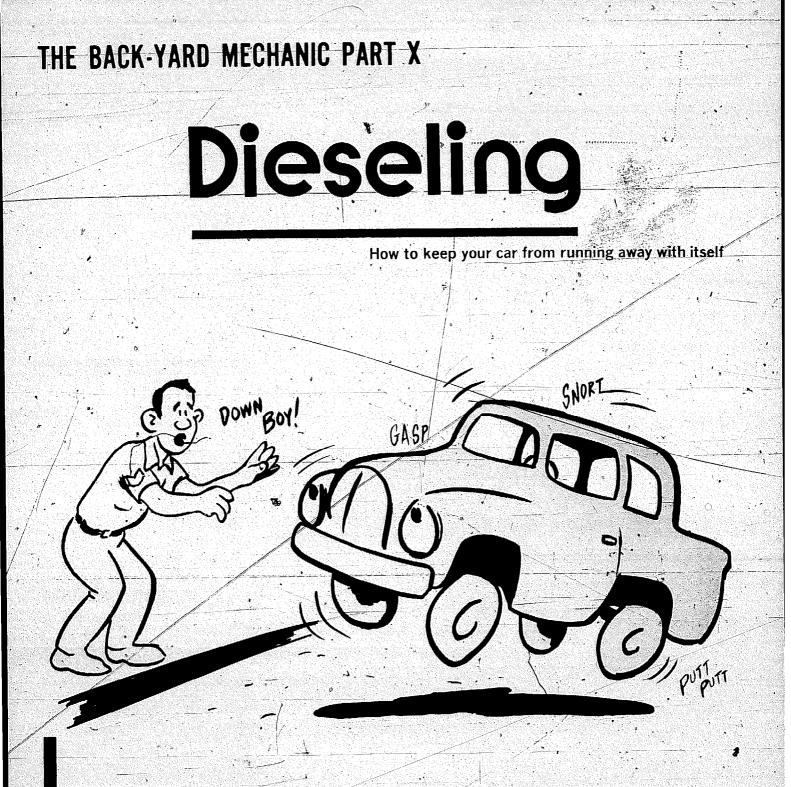
t's probably no surprise to most of you if your car runs for a few seconds after you switch off the ignition. "Dieseling." or "run on" as this condition is called. is rather common especially with 1968 and newer American cars.
