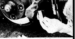
brakes are self adjusting—as the friction pad wears thinner, the piston comes farther out of its bore to maintain a proper seat between the pad and the disc. Therefore, each piston must be pushed back into its bore to create room to slide the new, thicker pad into the caliper.
