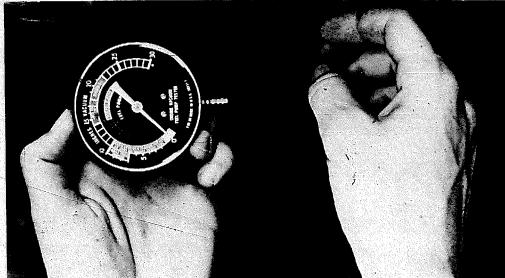
**To get accurate** vacuum readings, the gage must be attached to a primary source of manifold vacuum. The best installation procedure varies from engine to engine, but simply attaching the gage to the vacuum advance line at the distributor doesn't work.
