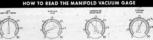
A line but steady reading generally indicates late ignition timing. If resetting the timing to specifications doesn't ima prove the reading, valve timing is incorrect.
