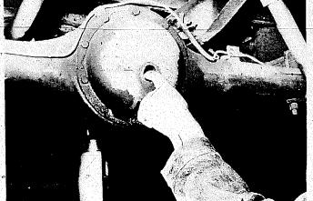
Check the standard transmission and differential fluid levels by removing the plugs located on the side or back of the housings. If the car is sitting level, the fluid should at least be even with the bottom of the hole. Your manual gives lubricant specifications.
