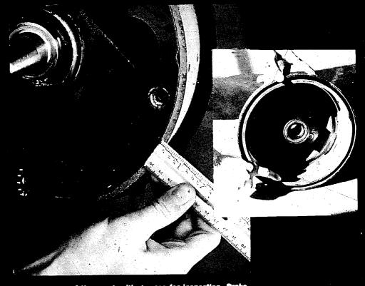
Braines are one of the most critical areas for inspection. Braine shoes should have at least 1/32-inch of lining above the rivets, or above the shoes on bonded linings. Disc brakes should also be measured for ped thickness—your owner's manual will give the recommended thickness. Brake drums should be evenly worn and free of large scratches or grooves. Worn drums can be machined and reused, but excessively or unevenly worn drums should be replaced.
