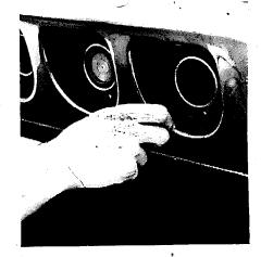
from the outer lens (see picture) Sometimes the bulb must be reached from under the body, as in the case of body side lights. Tail and back-up lights are usually accessible from the trunk.
