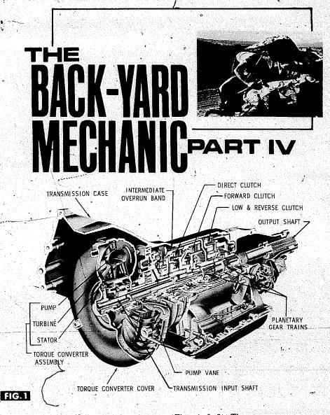
the engine. Inside its housing are three sets of blades known as the pump, stator, and turbine, immersed in light oil (transmission fluid) (Fig. 1). Energy passes from the engine through the fluid and the blades, and is transmitted as mechanical torque to the drive wheels by the output shaft. All three blade sets rotate together at cruising speed, providing maximum output with little slippage. At idle, the torque converter allows maximum slippage and very little torque output.
