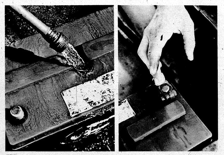
After washing, the battery should be kept clean and dry. After reinstalling the cables, lightly coat the tops of the terminals with petroleum jelly to prevent corrosion build-up.
