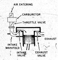
rig. 1 Idle: Throttle plate is closed—vacuum is high. Acceleration: Throttle plate opens (shown) allowing air to be drawn in—vacuum drops.
