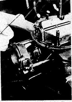
of the carburetor with this choke. The in-carb choke is characterized by the round thermostatic coil cover on the back or side of the carb.
