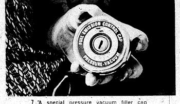
A special pressure vacuum filler cap must be used on all cars equipped with a fuel evaporative system.
