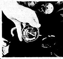
5 The temperature sensor is probably faulty if the snorkel valve doesn't open properly as the engine warms. Lift the air cleaner and check for vacuum at the line which runs from the engine to the sensor. If there is at least 8 psi, replace the sensor.
