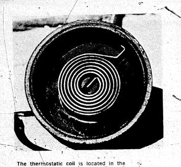
The thermostatic coil is located in the plastic cover on in-carb chokes. The coil is easily replaced if weak or seized.
