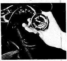
If the snorkel of a GM system fails to close when a cold engine is started, check for at least 8 psi of vacuum at the diaphragm unit. Low vacuum means a leaking hose or connection is causing the problem. If the vacuum is sufficient, replace the diaphragm.
