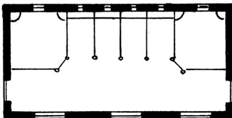
Fig. 91.—Ground Plan of Stable with Four Stalls and Two Boxes. Single row.
