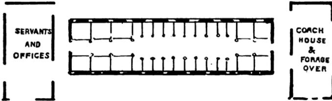
Fig. 93.—Ground Plan of Stable for thirty horses with ten loose boxes.
