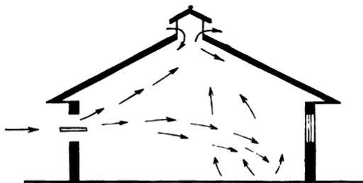
Fig. 6.—Direction taken by air currents with the windows open to windward.
