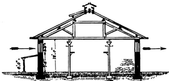
Fig. 1.—Transverse section of stable. Two horses are placed between opposite windows, heads to outer walls. The arrows indicate the direction of the wind.
