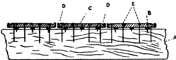
Fig. 86.—Open Board Roof. A, Frame of roof; B, studs driven in the frame to keep the boards, C, from touching it; D D, two grooves on either side of the boards to carry off the rain; E, long nails to secure the boards to the frame (Henderson).\*
