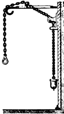
Fig. 116.—Collar Chain, with Spring Hook and Counterpoise.
