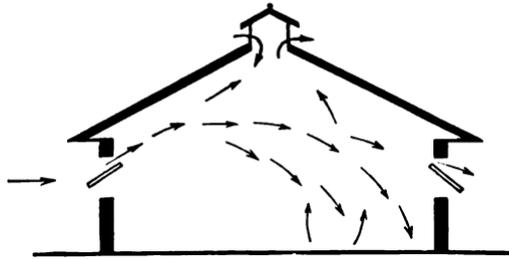
Fig. 9.—Direction taken by air currents when opposite windows are half open.
