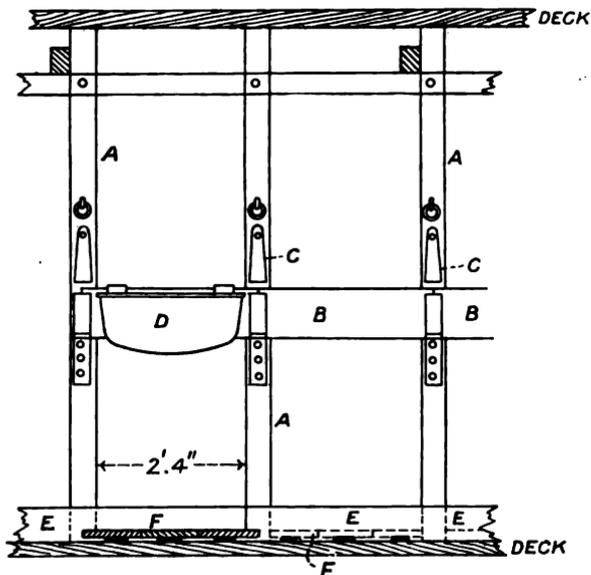
Fig. 211.—Front view of Horse Stall on Board Ship. A, front stanchions; B, breast bar; C, swinging stop; D, manger; E, front cant; F, platform.
