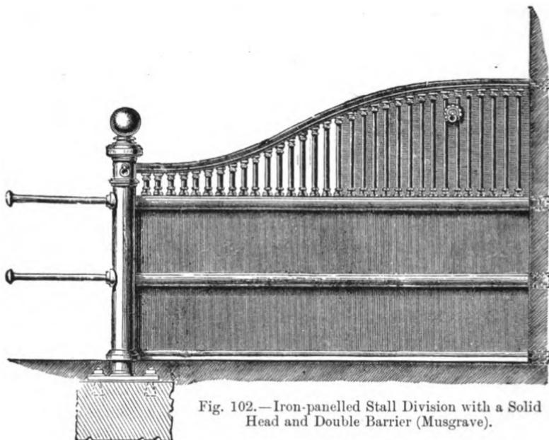
Fig. 102.—Iron-pannelled Stall Division with a Solid Head and Double Barrier (Musgrave).
