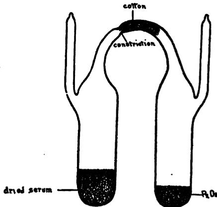
Fig. 69.—A tube used for the preservation of antitoxin by the Hygienic Laboratory of the Public Health and Marine Hospital Service: *a*, Serum scales, or antitoxin; *b*, phosphorus pentoxid, an active dehydrating agent (M. J. Rosenau, Bulletin No. 21, Hygienic Laboratory).
