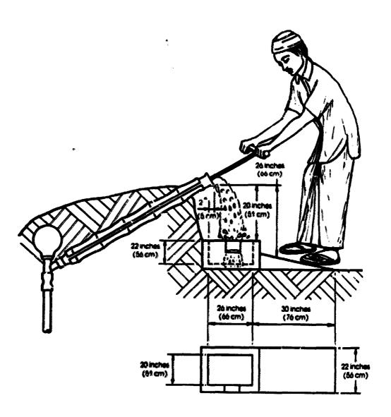
falls should be of such construction as to prevent erosion. Soil should be packed around the complete pump as near to the discharge end as possible.
