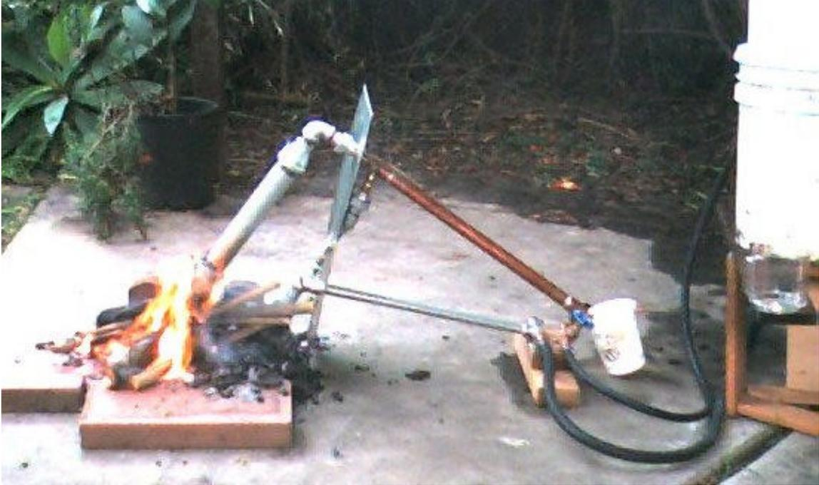
During operation most of the attention is on the fire and keeping it hot around the boiler pipe. The second most attention is on the water flow adjustment. Besides that the unit is nearly automatic and low tech.
