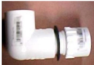
Feed throughs for the tanks were constructed of 1.25" PVC threaded pipe adaptors (see above). A hole was drilled in the side of the plastic tanks. A threaded male and female PVC pipe connector was screwed together with a rubber washer on each side of the tank. Silicon II was used to seal the connection.
