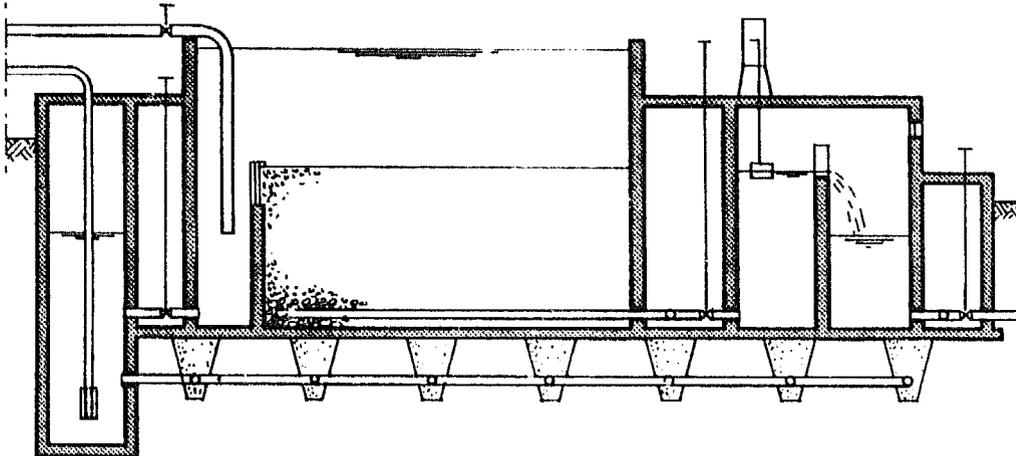
Figure 7.8: Drainage system underneath filter box
