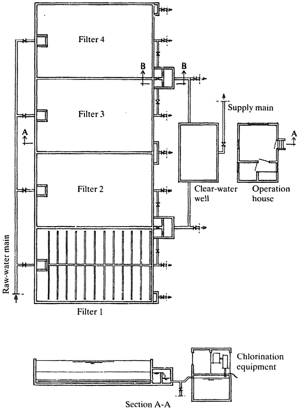
Figure 8.4: Design features of design example IV
