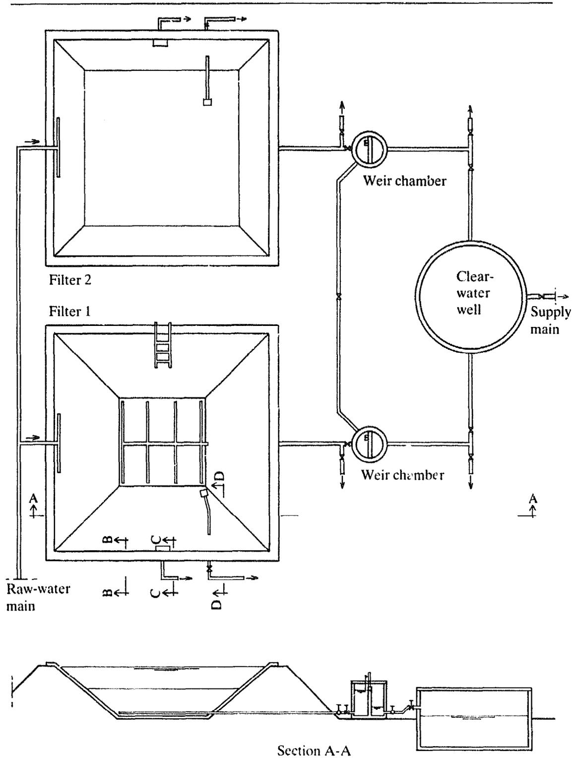
Figure 8.2: Design features of design example II
