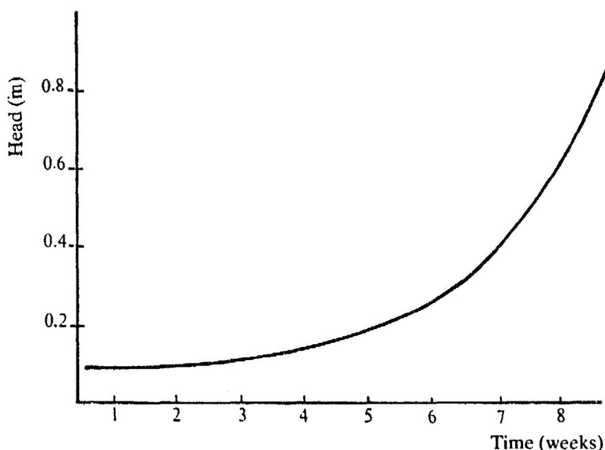
Figure 3.3: Development of resistance in the filter bed
