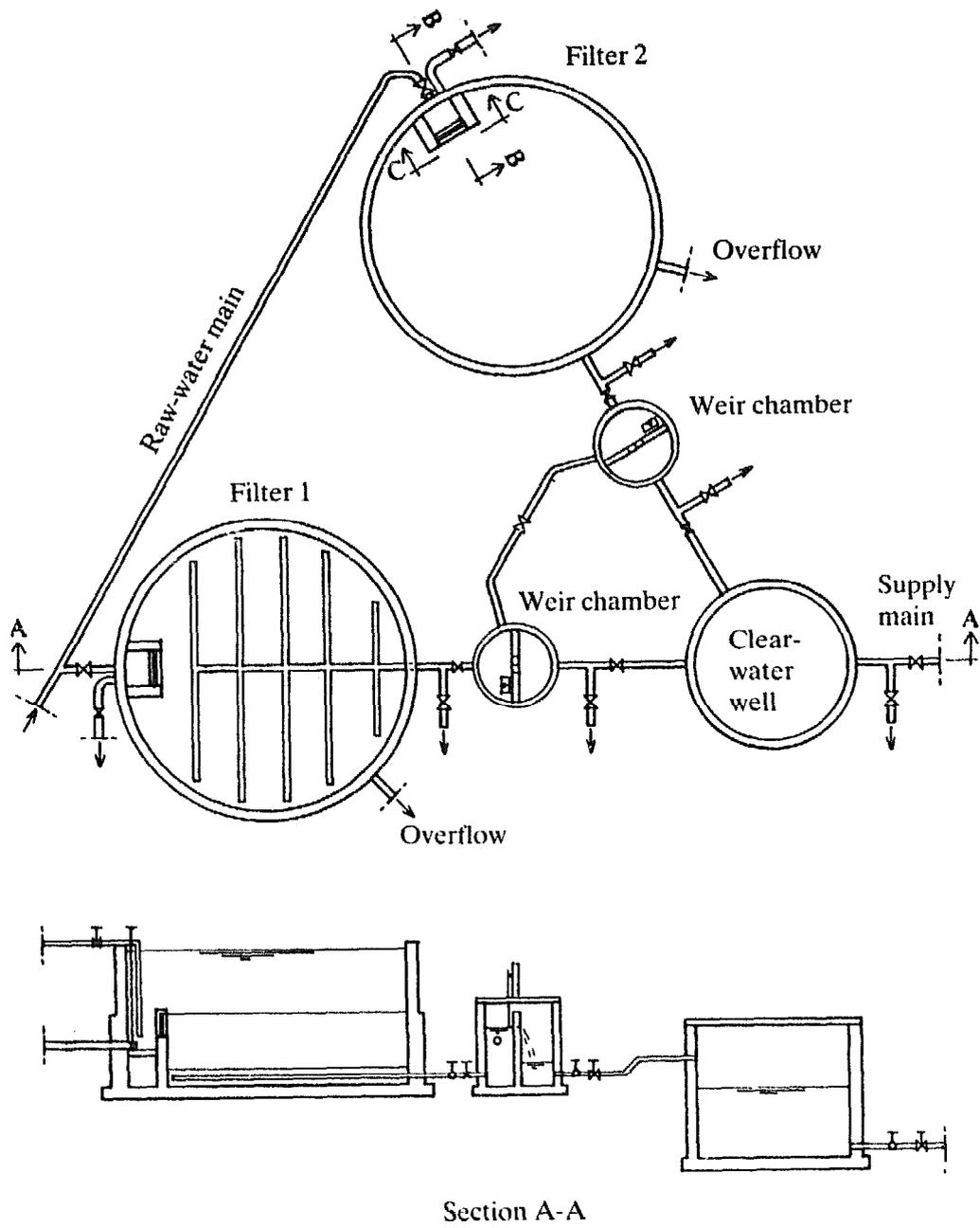
Figure 8.1: Design features of design example I
