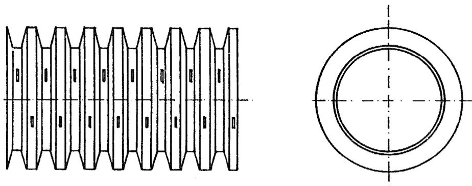
Figure 7.17: Underdrain system made of corrugated PVC pipe
