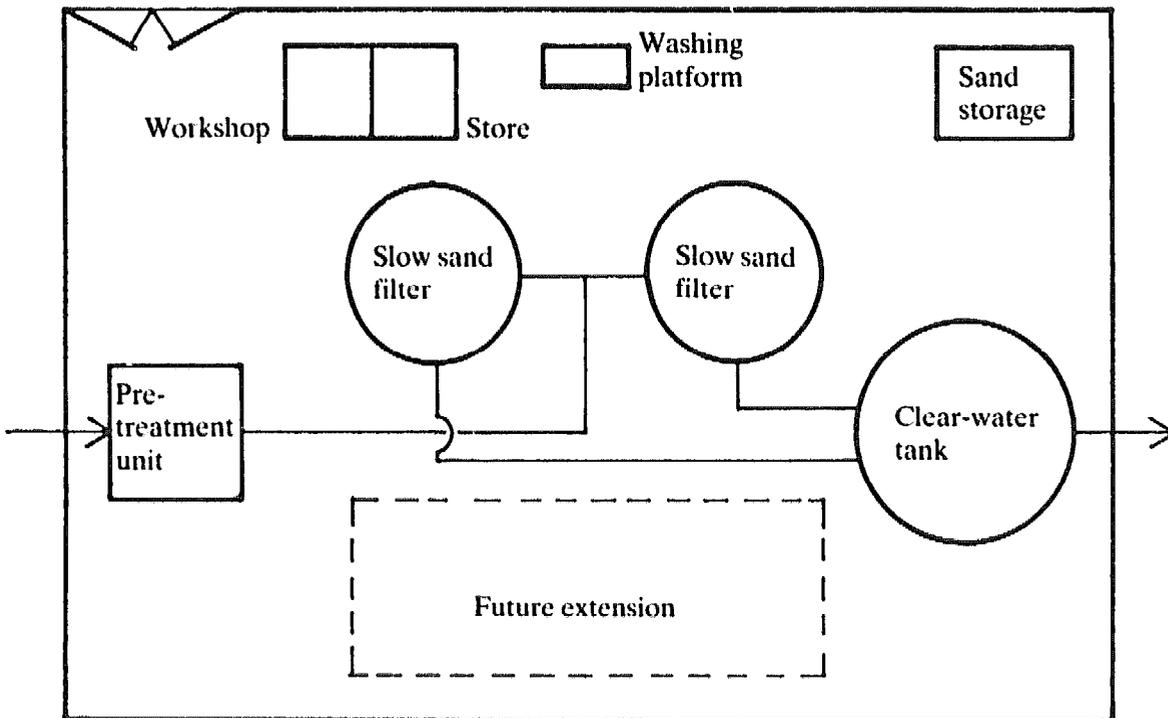
Figure 6.5: Possible layout of the water treatment plant
