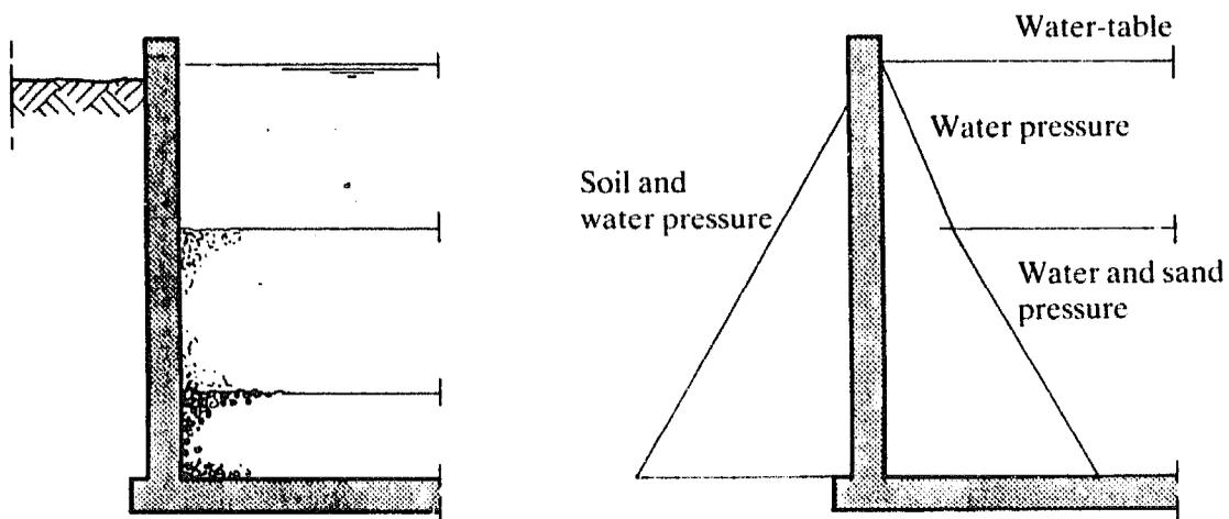
Figure 7.7: Pressure diagram for a wall of the filter box
