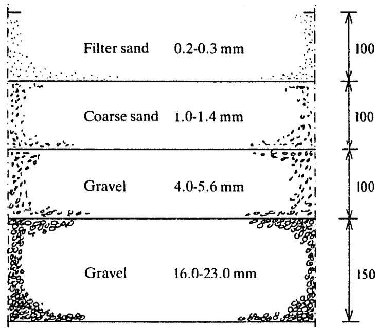
Figure 7.16: Filter medium support
