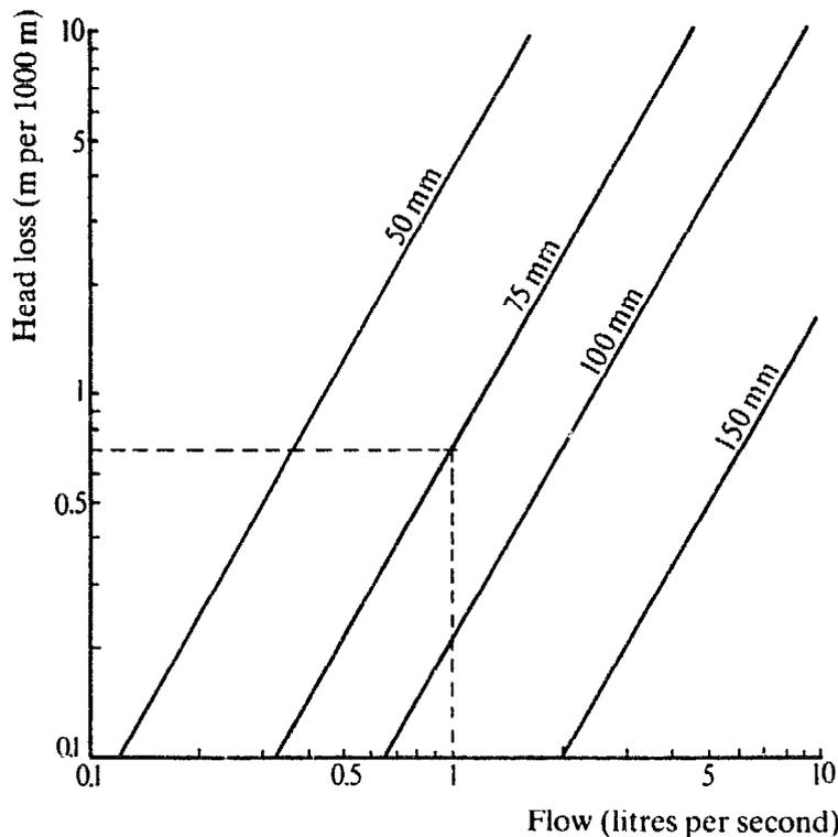
Figure 7.22: Head losses through friction in PVC pipes
