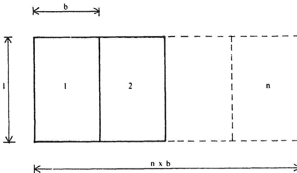
Figure 5.1: Layout of a filter plant with ( $n$ ) rectangular units
