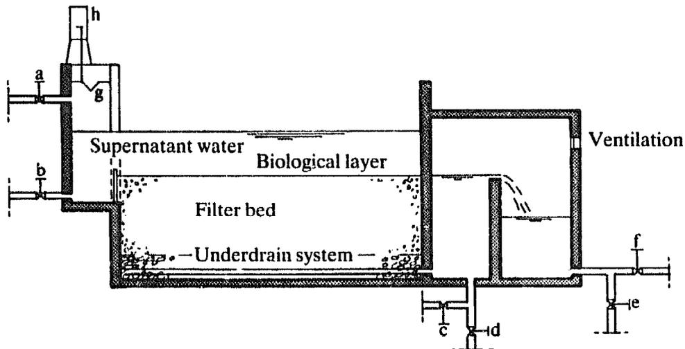
Figure 3.2: Basic components of an inlet controlled slow sand filter
