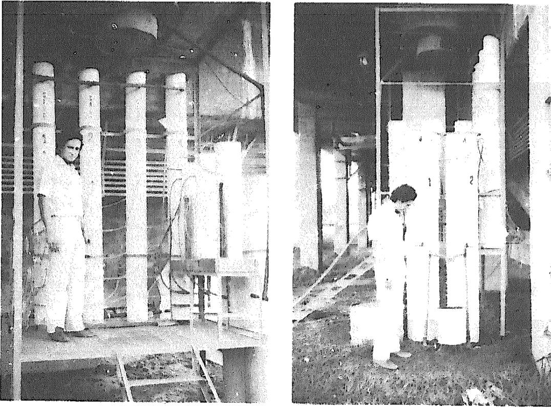
Figure 3.6: Slow sand filter pilot plant, Cali, Colombia
