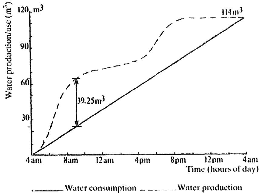
Figure 6.4: Accumulated water production and water use
