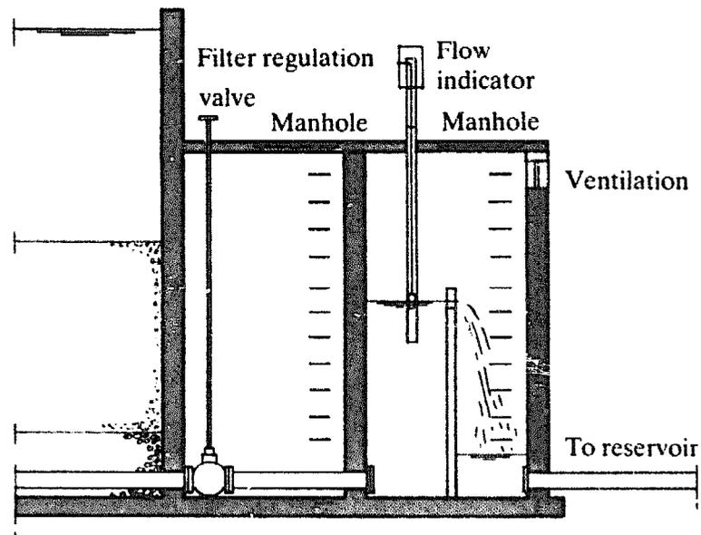
Figure 7.14: Outlet box of an outlet controlled filter
