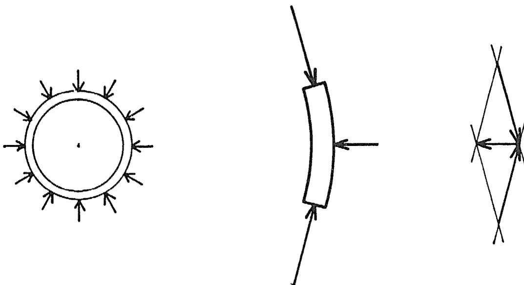
Figure 7.2: Principle of universal compressive and tensile stresses
