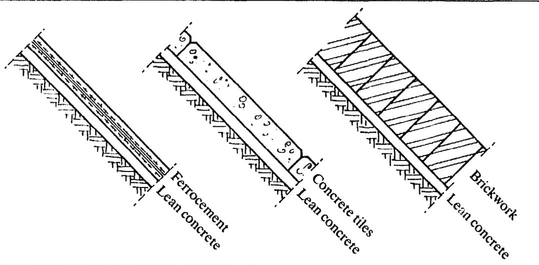
Figure 7.12: Various linings for sloping wall filters
