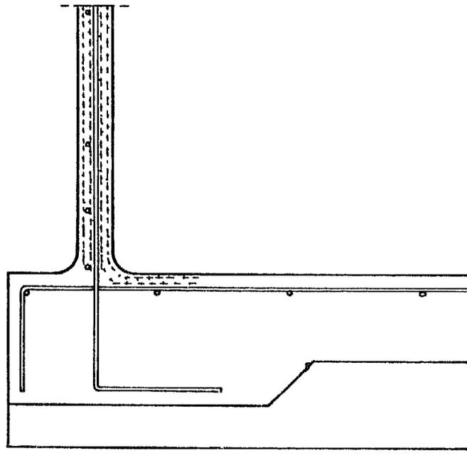
Figure 7.9: Wall-floor connection in ferrocement and reinforced concrete
