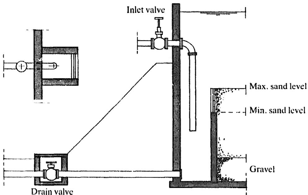
Figure 7.13: Inlet structure
