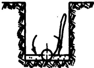
2. Tamp soil under pipes and between pipeline and trench wall at both side. Water tamping may be used where drainage is good.
