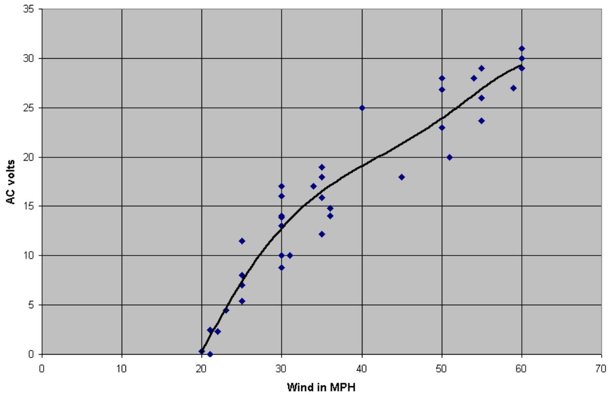
Other small fans may work better. If one has a way to produce a strong AC magnetic field one should be able to lower the field strength of the PM. Will need to take it apart to do this. Most have a metal shield around the magnet so that attempting this from the outside doesn't work. I tried it. If the PM field is reduced it should start at a lower speed.
