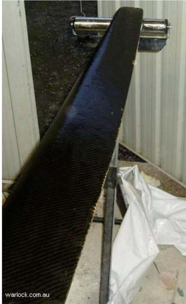
Figure 9. Blade after sanding the carbon fibre
