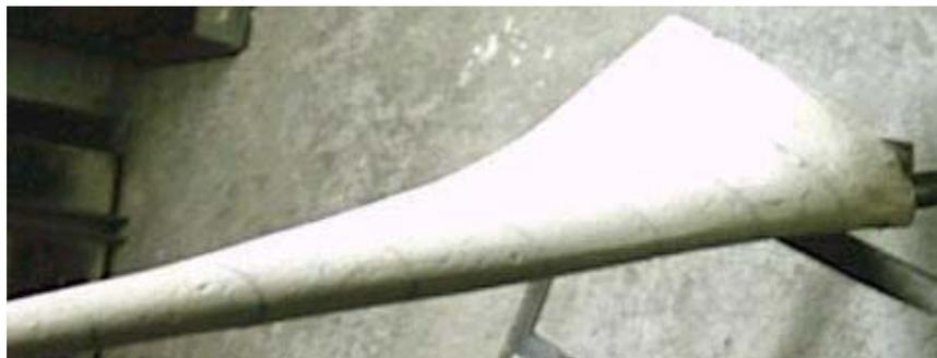
Figure 5. Polyurethane foam blade after sanding
