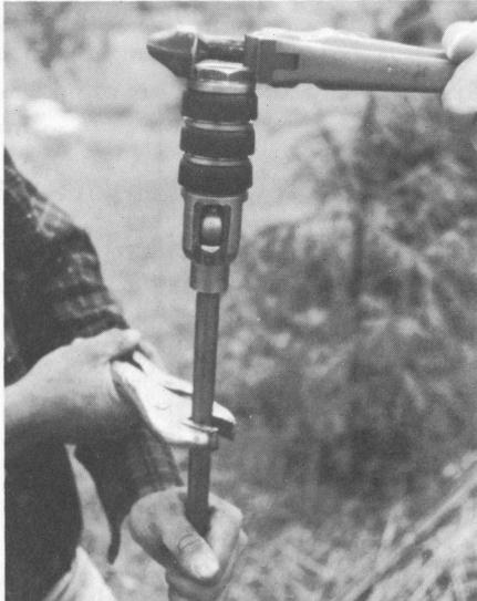
*Figure 5.5. Attaching the plunger to the pump rod.*
