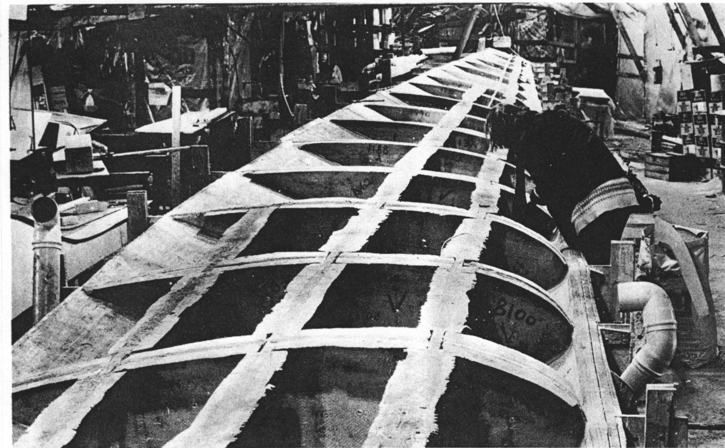
**Wing-Sections with sawn-out "Flamingo"- Polystyrol blocks.**
