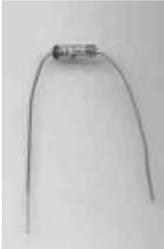
A diode (also called a rectifier) only allows current to go in one direction. Current flowing in the opposite direction is stopped. Think of a diode as a one-way valve for electricity. Diodes are rated as to how much current they can handle, and the maximum amount of reverse voltage they can withstand (this is called the Peak Inverse Voltage, or PIV).
