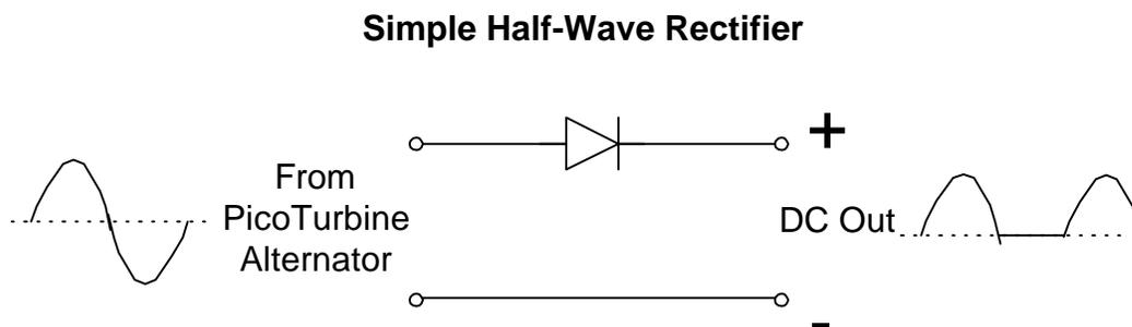
The circuit uses only a single diode, which you will recall, acts like a one-way valve for electricity. Sometimes two diodes, one in each direction, are used in half wave rectifiers.
