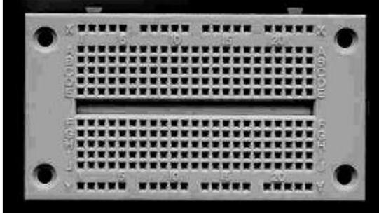
The solderless breadboard allows you to quickly set up circuits without having to make solder connections. This is faster and much safer in a classroom setting. The breadboard is marked so that rows have a number and columns have a letter. This kit will tell you to make connections using a combination of a letter and number. For example, “place a diode from A3 to A5”. This would mean place the unmarked side of the diode in A3 on the breadboard and the marked side in the A5 hole.
