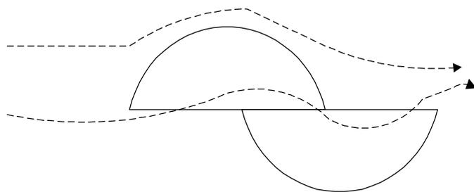
With the wind coming from the left side of the page, this shape assumes a simple air foil-like configuration, causing some lift to aid the rotation of the turbine. It is also this effect that allows the turbine to start up even if it has this profile from a dead stop. However, torque is minimal in this position relative to the wind.
