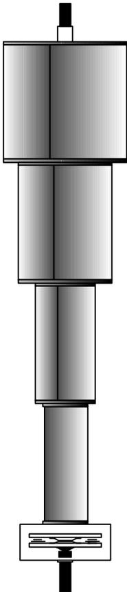
If you have access to Teflon tape, it is desirable to clean the outer surface of the 1" pipe and apply several rings of tape. The tape should be oriented such that the rotation of the blades will tend to wrap it tighter rather than to rub against the outer edge of the tape and cause it to unwrap. Several rings of tape should be placed near the top and the bottom sections of PVC pipe, where the most friction occurs.
