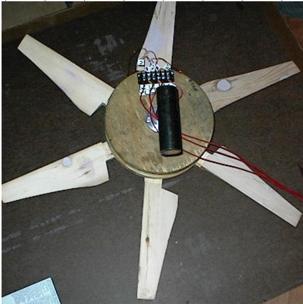
Still only 30" in diameter, testing was done in a 14 mph wind and the results are coming out good. Unloaded the blades run around 720 rpm and with a load 570 rpm. Using a slightly dead battery with a 50 watt load its making 11.75 volts at 1.7 amps ( total of 19.9 watts ). The total available watts for that area of blade is 77.78 so that makes the overall efficiency of around 25%. It will make about 170 watts in a 30mph wind and the efficiency drops to around 22%. Still just over 13 amps at
