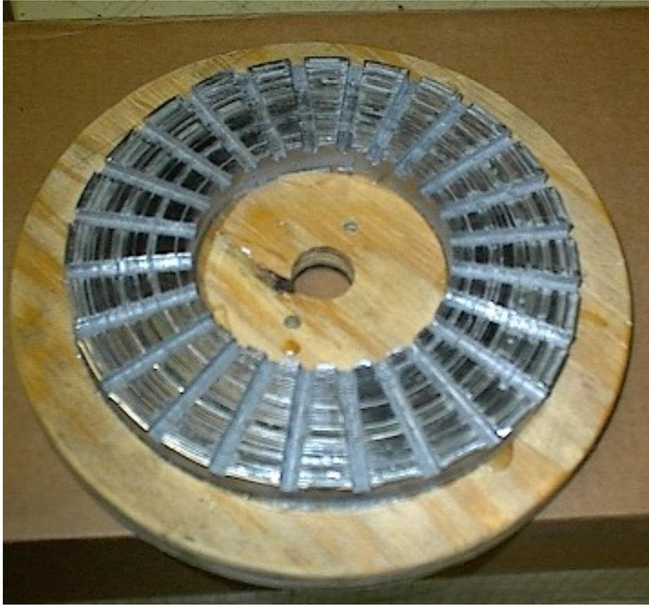
**There is 60 feet of 3/4" steel in this stator. The stator is 8" in diameter and 2" wide. Below show the winding in process...**
