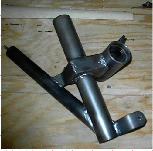
All bead blasted and ready for paint. Here you can see the alternator lower mount at the bottom and the upper mount in the left hand picture. The main shaft head was machined to accept a standard 1" tapered roller bearings for a small trailer.
