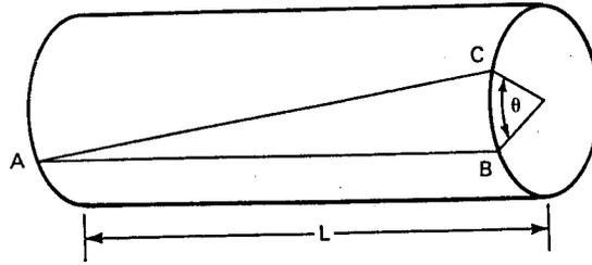
Figure 22: Shaft twisted under an applied torque.
