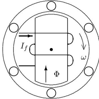
Figure 9: Three-phase generator
