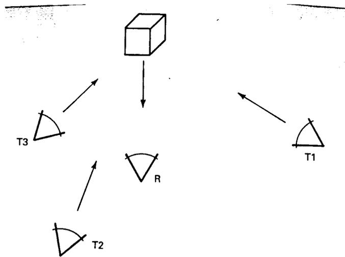
Figure 8: Doppler acoustic radar configuration.
