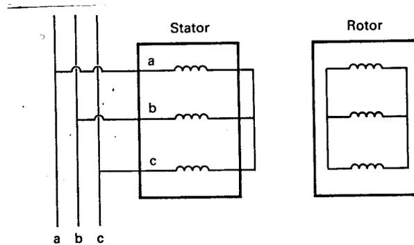
Figure 16: Wiring diagram for a three-phase induction motor.
