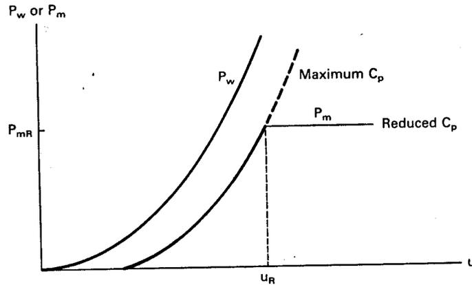
Figure 7: Shaft power output of a variable-pitch turbine.
