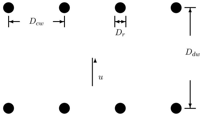
Figure 1: Dimensions of Turbines in a Windfarm
