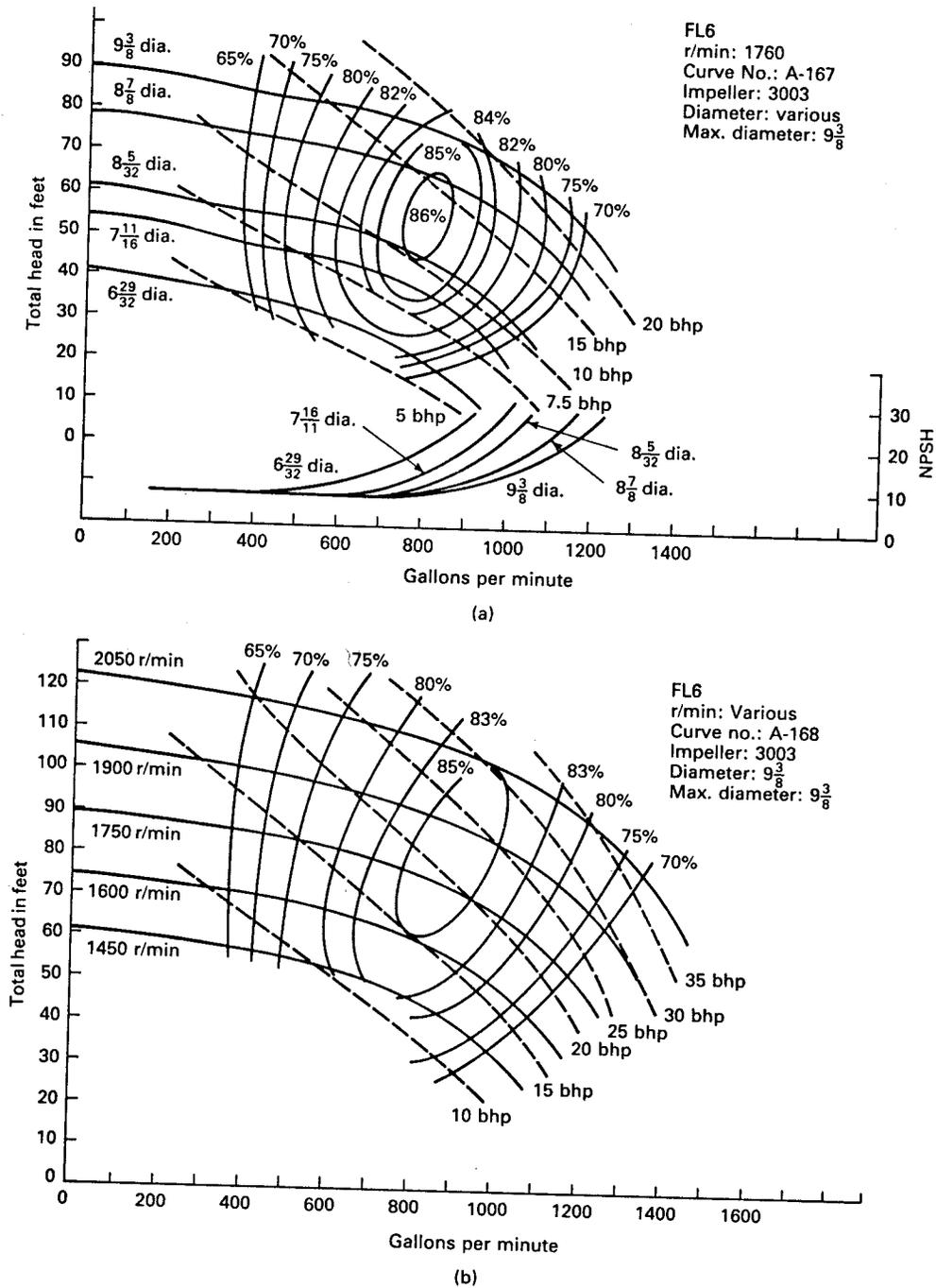
Figure 7: Pump performance curves for Jacuzzi Model FL6 centrifugal pump: (a) head-capacity curves as the impeller size is varied; (b) head-capacity curves for a  $9\frac{3}{8}$ -in.-diameter impeller at variable speed. (Courtesy of Jacuzzi Bros. Inc., Little Rock, Arkansas.)
