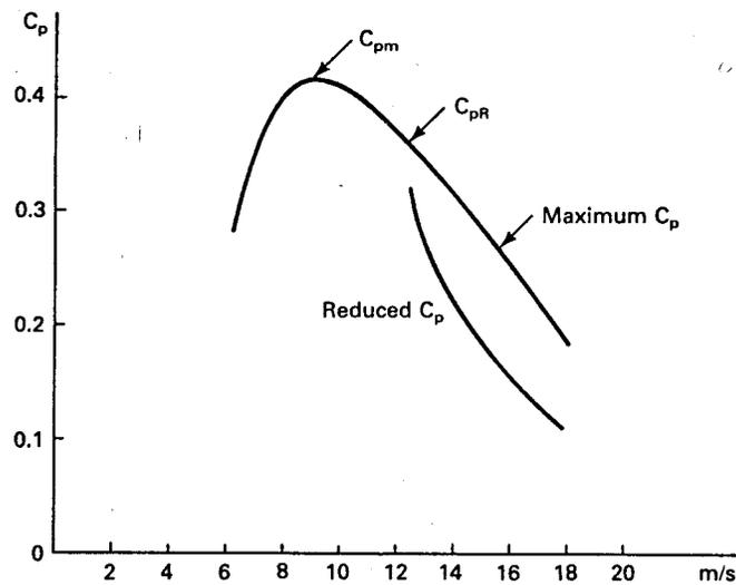
Figure 8: Coefficient of performance versus wind speed for MOD-2.
