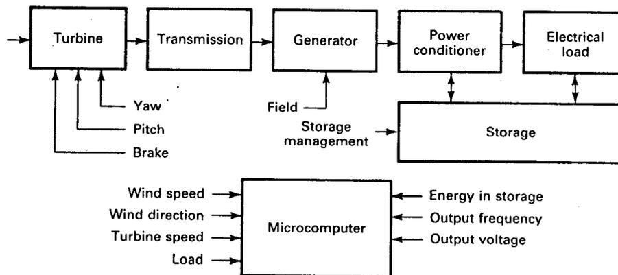
Figure 1: Block diagram of asynchronous electrical system.
