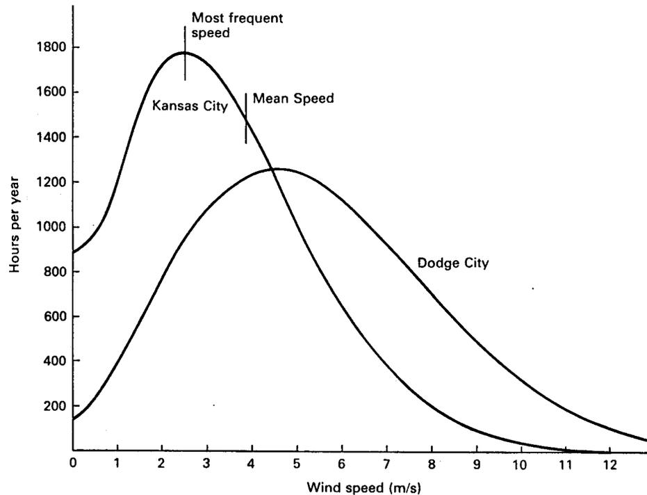
Figure 7: Speed-frequency curves, 1970
