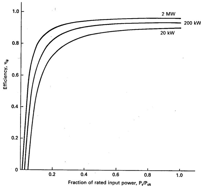
Figure 14: Generator efficiency for three generator sizes.
