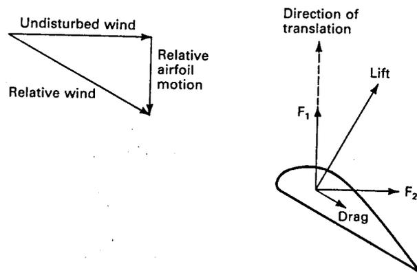
Figure 4: Lift and drag on a translating airfoil.
