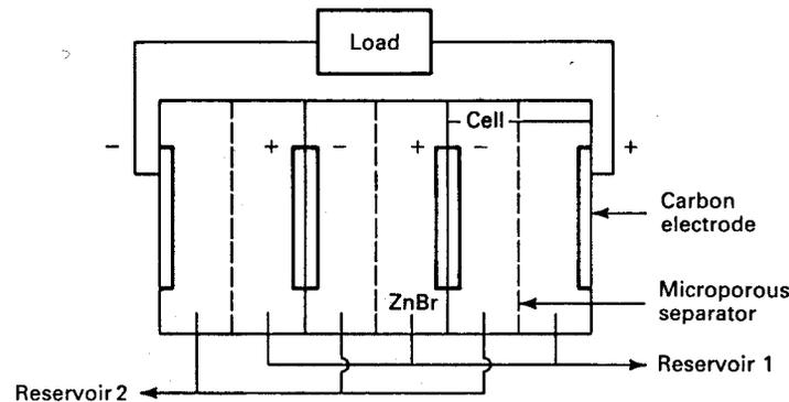
Figure 12: Diagram of a zinc bromide battery.
