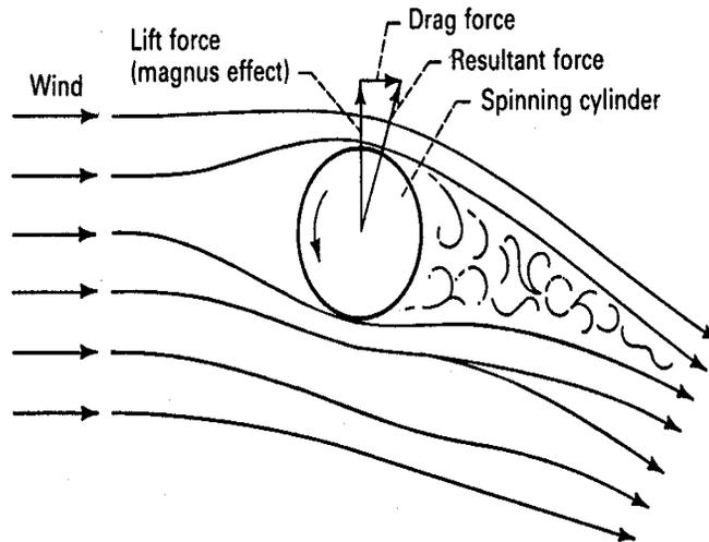
Figure 9: Magnus force on a spinning cylinder.
