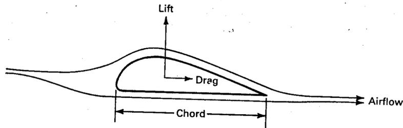
Figure 3: Lift and drag on a stationary airfoil.
