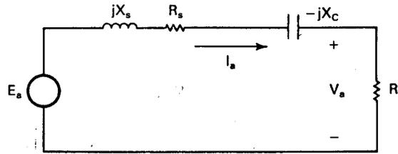
Figure 9: Series resonant circuit for a PM generator.
