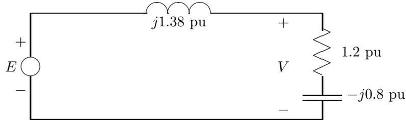
Figure 14: Per phase diagram for example problem.
