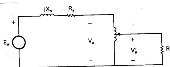
Figure 6: Load adjustment with a variable autotransformer.
