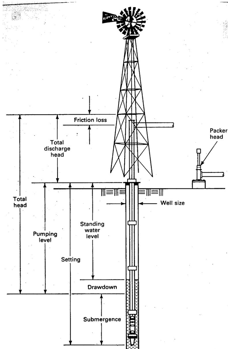
Figure 1: Aermotor illustration of key water pumping terms.
