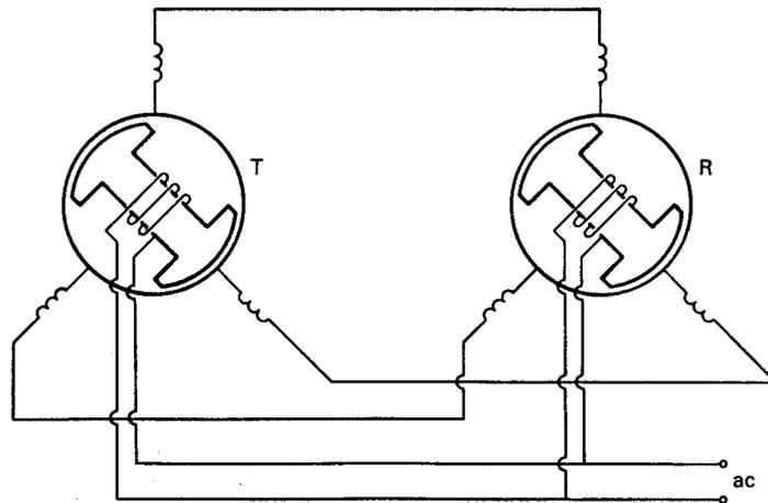
Figure 11: Synchro wind direction transmitter and receiver.
