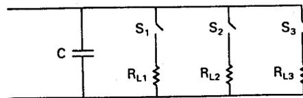
Figure 17: Minimum capacitive and resistive loads for a self-excited induction generator.
