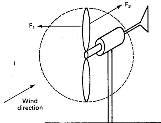
Figure 5: Aerodynamic forces on a turbine blade.
