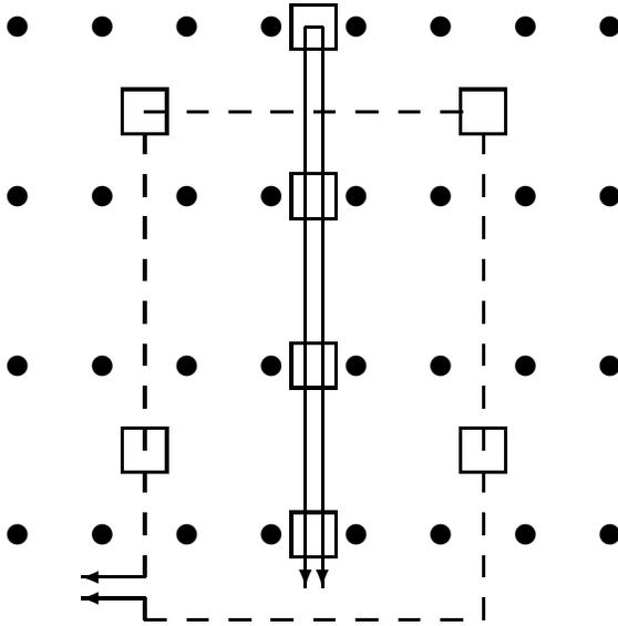
Figure 4: Trench lengths for distribution voltage wiring for 32 turbines in 4 rows, for both  $1 \times 8$  and  $2 \times 4$  low voltage configurations.
