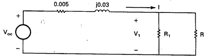
Figure 15: Single-phase transformer connected to two resistive loads.
