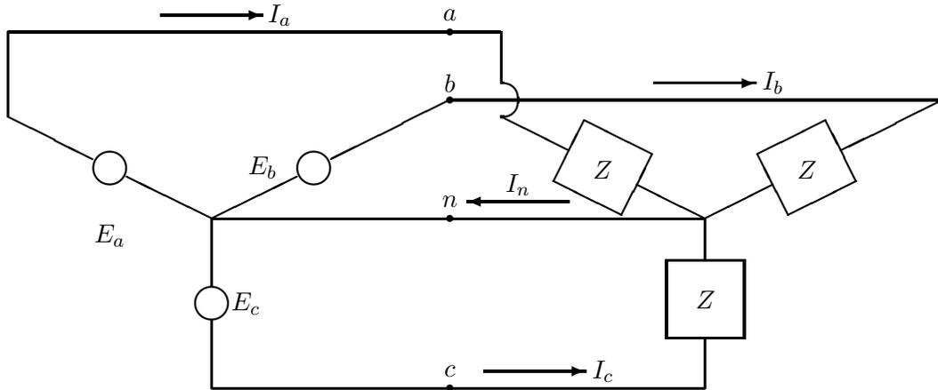
Figure 8: Balanced three-phase wye-connected source and load.
