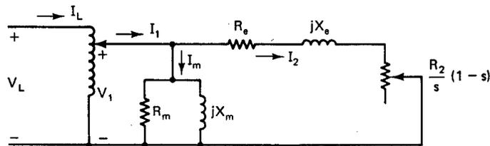
Figure 21: Circuit for autotransformer start of induction motor.
