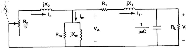
Figure 11: Single-phase equivalent circuit of self-excited induction generator.
