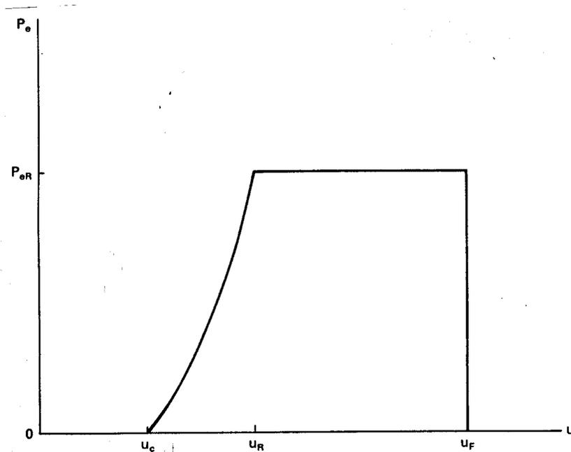
Figure 16: Model wind turbine output versus wind speed.
