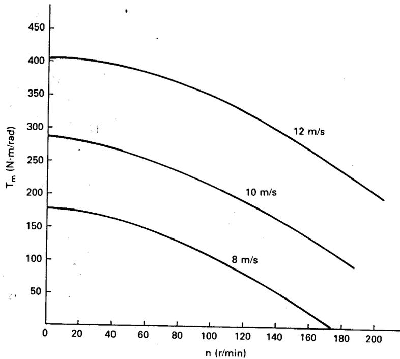
Figure 31: Torque versus rotational speed for Savonius turbine: radius 0.88 m; area 22 m<sup>2</sup>.
